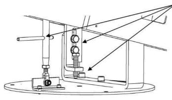
There are three points of adjustment. For leveling of the target trajectory, the right side support leg is adjustable. See the two lock bolts and a height adjustment bolt, which can be adjusted to achieve a perfectly flat trajectory. The vertical adjustment (target height) is simply done by a turnbuckle. Further adjustment can be made by loosening the bolt at the base plate. This will allow rotation of the machine to either side for wind adjustment.
