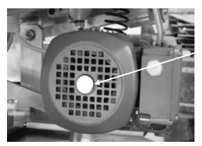
On the MTD500, the vertical motor is used to adjust the height of trajectory. Stop the vertical oscillation at an approximate level, then you may "fine tune" the height by turning the knurled bolt head at the back of the motor.
