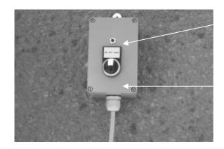
Remote control box with its flashing LED, to indicate that the launcher is on.
