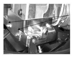
Adjusting the drive belt tension may be done by loosening the 2 fasteners at the front of the reduction gear bracket, and the 3<sup>rd</sup> at the rear of the bracket as shown, then by tightening up or (backing off) the tension bolt, as shown, will move the entire gearbox/motor in/out, thus changing the belt tension.
