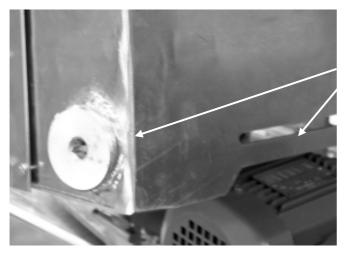
Setting the target throwing distance is easily done by the multipurpose tool a 3/8" drive ratchet. A spring tension indicator as shown, is very helpful when changing from single to double throw. Silmply insert the ratchet and "turn up" the spring tension to desired distance of 50 yards for single target, mark the position of the
