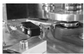
The adjustment of the launching arms stopping point (ready to fire position) is done via the micro switch, which is located at the magazine drive member. By loosening the set screws (2 ea.) in the inner bearing collar (race) about 11/2 turn, (use a 3 mm Allen tool) the collar may now be
